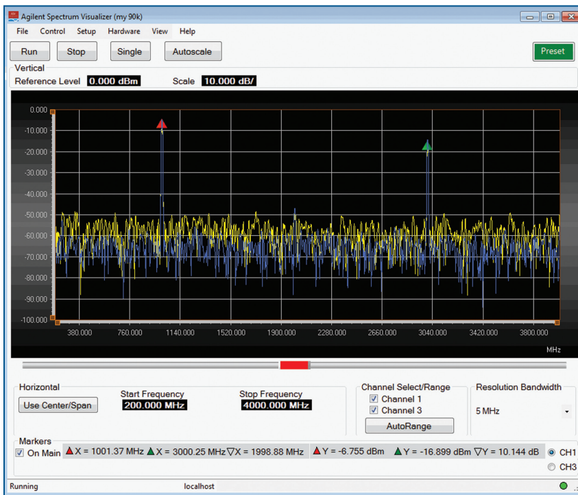
Figure 6: Using the marker functionality in the ASV software to determine the harmonic attenuation of the third harmonic relative to the fundamental frequency
